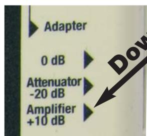
When the preamplifier is connected, set the "Adapter" switch of the HF-Analyzer to "Amplifier +10dB" (See picture on left). This activates the integrated automatic conversion feature of the HF-Analyzer. The true signal strength value can be read from the display without any manipulation. The vertical line on the left side of the display indicates the correct measuring unit.
