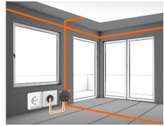
The grounding straps must be pressed down tightly to adapt perfectly to the underground. Mounting: Cross all areas once and connect them with each other, starting from GW / GB. The strap can be sticked under the baseboard if there are no doors.
